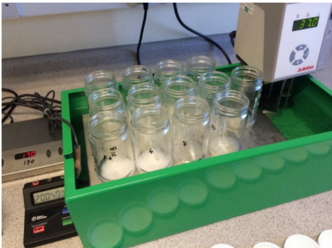
Figure 4. Picture showing a 2mag Mixdrive 15® submersible magnetic stirrer in a custom made water bath (Megazyme water bath (cat. no. D-TDFBTH )). This allows stirring of 15 samples at controlled speed (170 rpm) and 37°C.
