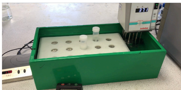
Figure 2. Incubation Method 1. Samples (~ 0.5 g) in 20 mL of buffer plus enzymes in 30 x 84 mm polypropylene tubes in a designed polypropylene tube holder (Megazyme cat. no. D-PPTH) on a 2mag Mixdrive 15 ® submersible magnetic stirrer in a custom made water bath (Megazyme cat. no. D-TDFBTH ).
