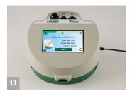
Add 400  $\mu L$  sample from the red dilution cup to the back of the Raptor cartridge. Reader will start automatically
