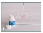
Add 1000  $\mu L$  of sample diluent to the red dilution cup and mix up and down 5 times
