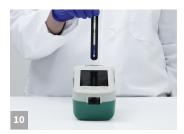
Insert strip into the Raptor° Solo cartridge. Insert cartridge into the reader.
