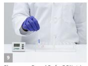
Place a new Reveal Q+ for DON strip into the sample cup. Set a timer for 3 minutes.
