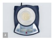
Obtain a representative sample. Grind and weigh out a 10 g sample.
