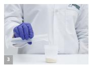
Add 100 mL of distilled or deionized water to the sample.
