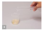
Add 100 mL distilled or deionized water to the sample.\*
