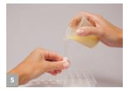
Allow to settle, then filter collecting a minimum 3 mL filtrate.
