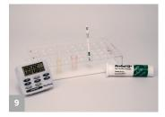
Place a new Reveal for T-2/HT-2 strip into the sample cup. Set a timer for 6 minutes.
