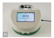
Add 400  $\mu$ L sample from the red dilution cup to the back of the Raptor cartridge. The reader will start automatically.
