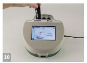
Insert the cartridge into the Raptor reader. Select Curve 1 or Curve 2 depending on matrix.
