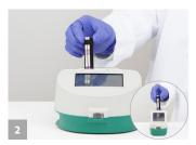
Insert the cartridge containing the test strip into any of the 3 ports within the Raptor Integrated Analysis Platform or single port of the Raptor Solo.
