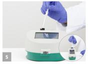
Pipette slowly 0.4 mL milk sample at the back of the cartridge. Press next. The analysis will take place automatically.
