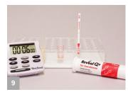
Place a new Reveal Q+ for Zearalenone strip into the sample cup. Set a timer for 6 minutes.
