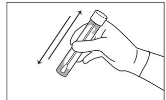
**8** In the lab, vigorously shake or vortex the swab for 10 seconds, to release bacteria from the swab tip.
