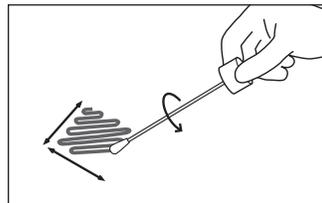
**6** Repeat Step 2. Change direction 45° and aseptically swab the same sampling surface while rotating the swab.
