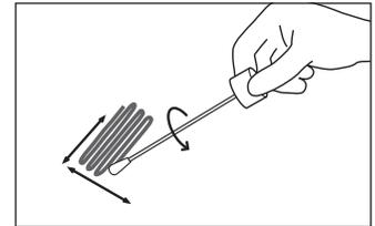
**4** Repeat Step 2. Change direction 90° and aseptically swab the surface while rotating the swab.
