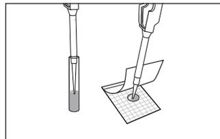
**10** Using a pipettor with a sterile tip, draw 1 mL from the tube and dispense onto a 3M Petrifilm Plate. Repeat for additional plates as needed.
