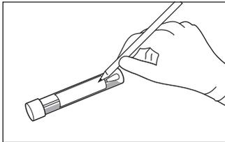
**1** Label the 3M Swab Sampler. Unscrew the cap from the tube and aseptically remove the swab from the tube.
